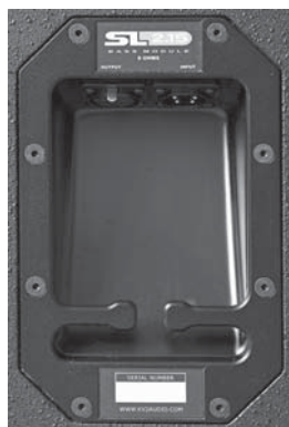
SL2.15 rear panel (cable connection to SL3000 unit Amplifier/Controller)
