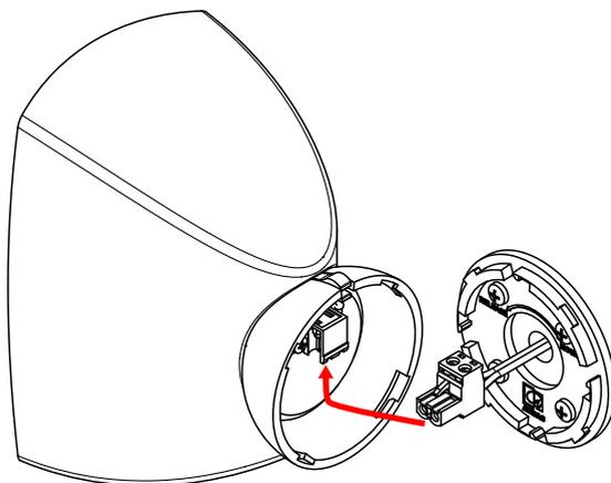
**Mind the polarity markings when wiring the loudspeaker cables.**
